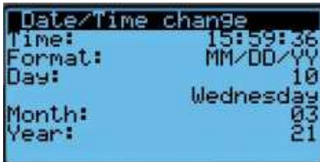
FIGURE 35 Setting Controller Date and Time
