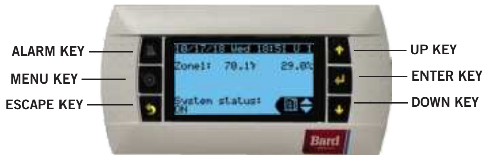
FIGURE 34 LC6000 Controller Display and Interface (Status Screen Shown)
