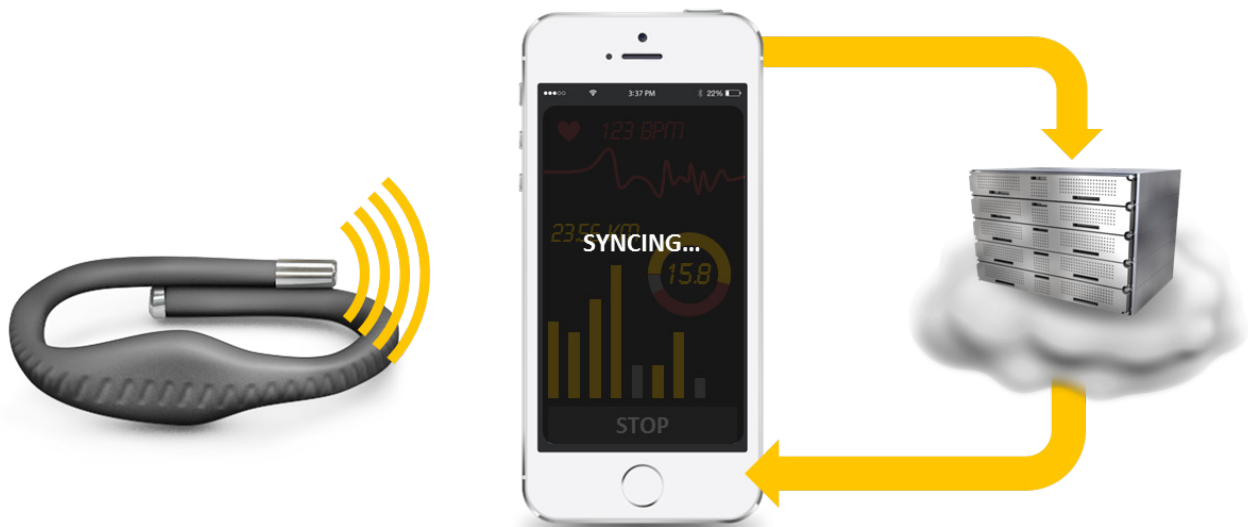
Figure 8. Self-tracking system model using a device, smartphone, and cloud-based server
