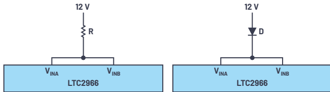
Figure 5. Possible reverse voltage protection methods for LTC2966.
