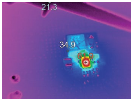
Figure 7. The 3\text{ mm} \times 4\text{ mm} LT8636 in a 13.5 V to 5 V/4 A constant load plus a 4 A pulsed load (10% duty cycle) thermal picture showing temperature rise.
