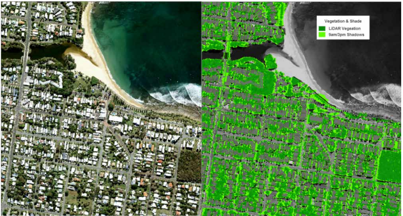
Figure 5: Shade is calculated using tree height and time of day within mapping software. The left image shows standard aerial photography, the right image, a LIDAR derived vegetation map with trees (non-ground vegetation) in dark green, and the 9am/3pm summer shadows in light green.
