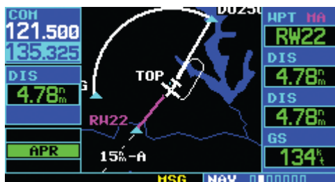
Figure 6-47 Final Course Segment
