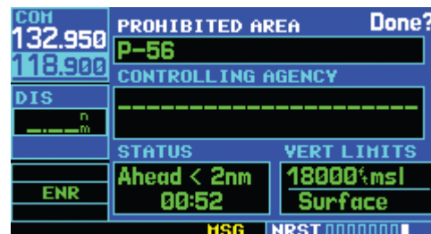
Figure 8-37 Airspace Page for Prohibited Area
