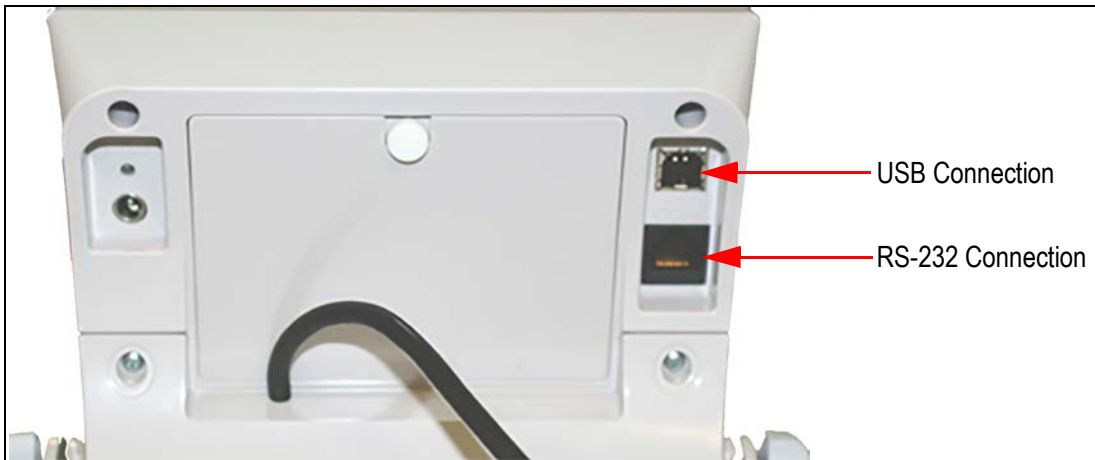
Figure 4-3. USB Connection Port
