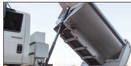
Mailhot® multi-stage, double-acting, nitrided cylinder, trunnion-mounted hoist
