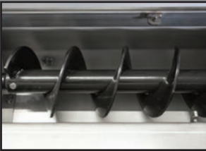
Heavy duty 9" auger for 92450SSA 6" auger for all other models
