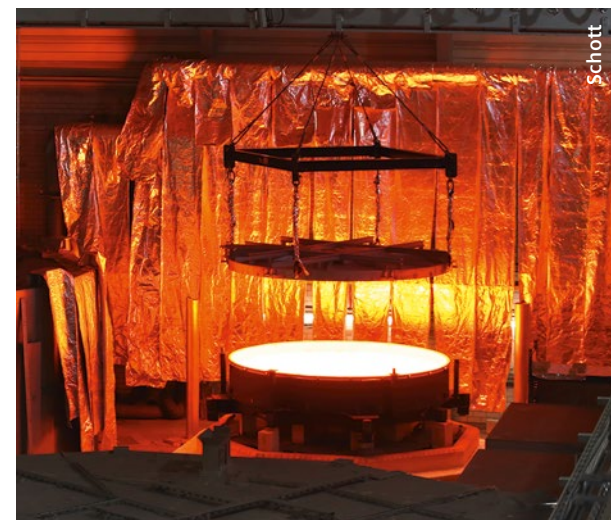
Building the mirror substrate for the world's largest optical telescope: The photo shows the mold being opened in the Schott cooling hall.
