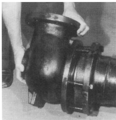
6. Slip new Shoe in place being careful not to damage Bottom Seat Ring O-ring.
