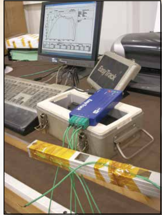
Cure Oven Temperature Test During the cure process oven air temperatures and part temperatures are monitored frequently to ensure proper curing of powder coating.
