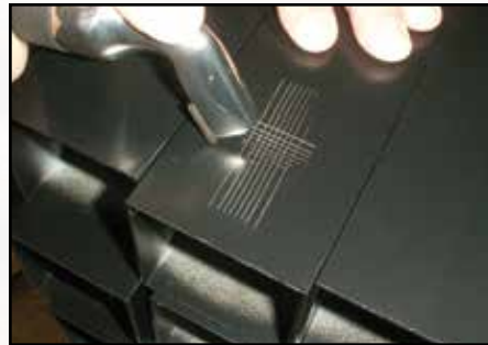
ASTM D3359 Crosshatch Test Hourly crosshatch testing is completed per ASTM D3359 to test coating adhesion.
