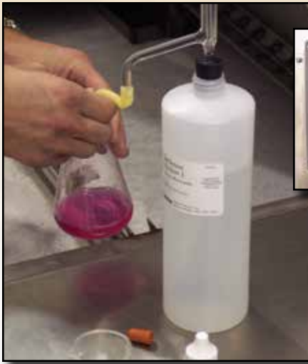
Automated Chemical Test Pretreatment chemicals are monitored and added automatically. Titration is checked manually twice per shift.
