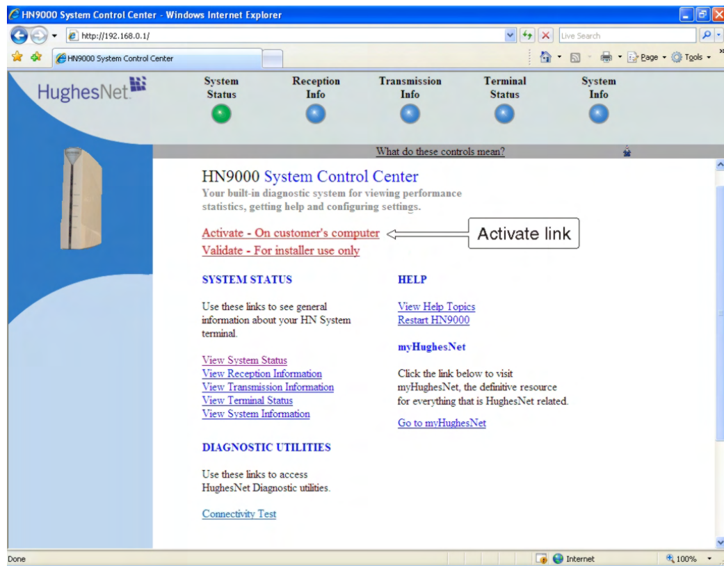
Figure 33: Activate link on the System Control Center home page
