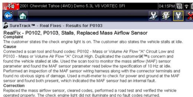
Figure 6-5 Related Real Fixes Screens
