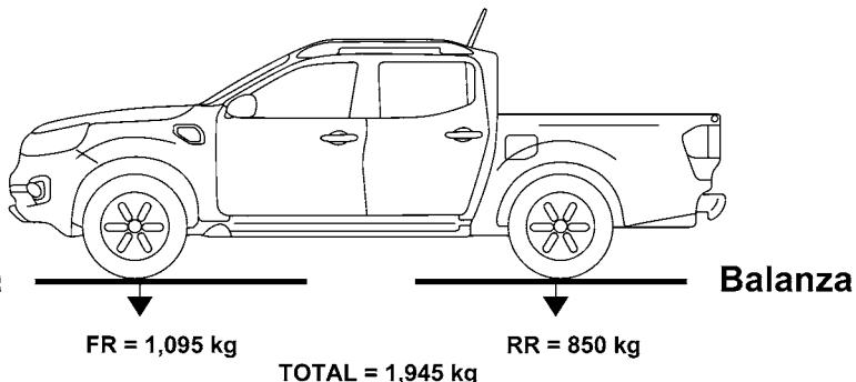
$$\begin{aligned} \text{RCC}_T &= \text{GVWR, peso medido} \\ \text{RCC}_T &= 2,820 \text{ kg} - 1,945 \text{ kg} \\ \text{RCC}_T &= 875 \text{ kg} \end{aligned}$$
