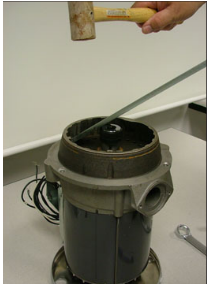
Figure 12. Removing Stationary Shredder
