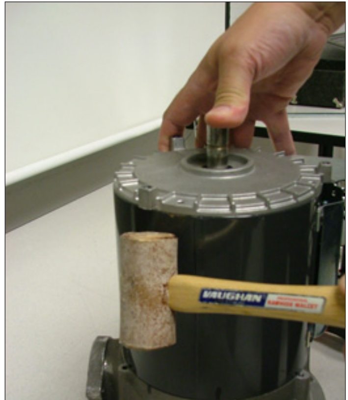
Figure 30. Marking and Removing Lower End Framer
