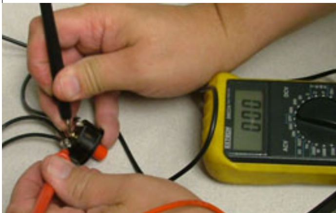
Figure 24. Testing Overload Protector
