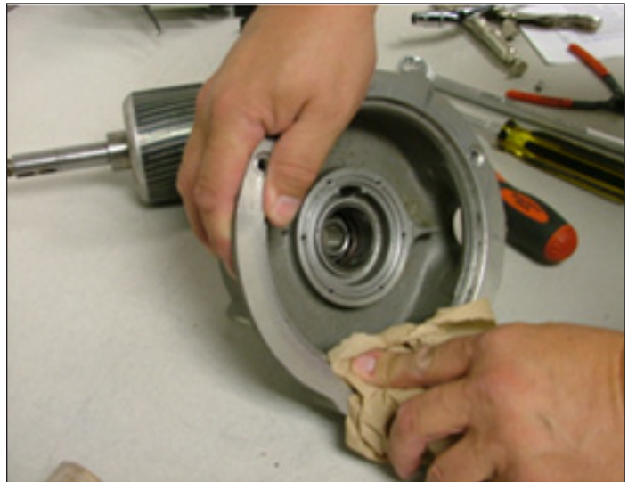
Figure 21. Cleaning Upper End Bell
