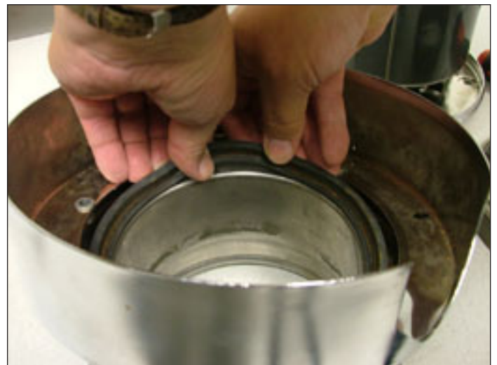
Figure 11. Replacing Shredder Gasket
