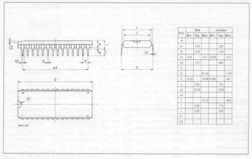
Figure 8 : MK48S74 28 Pin Plastic DIP (N) 300 MIL.
