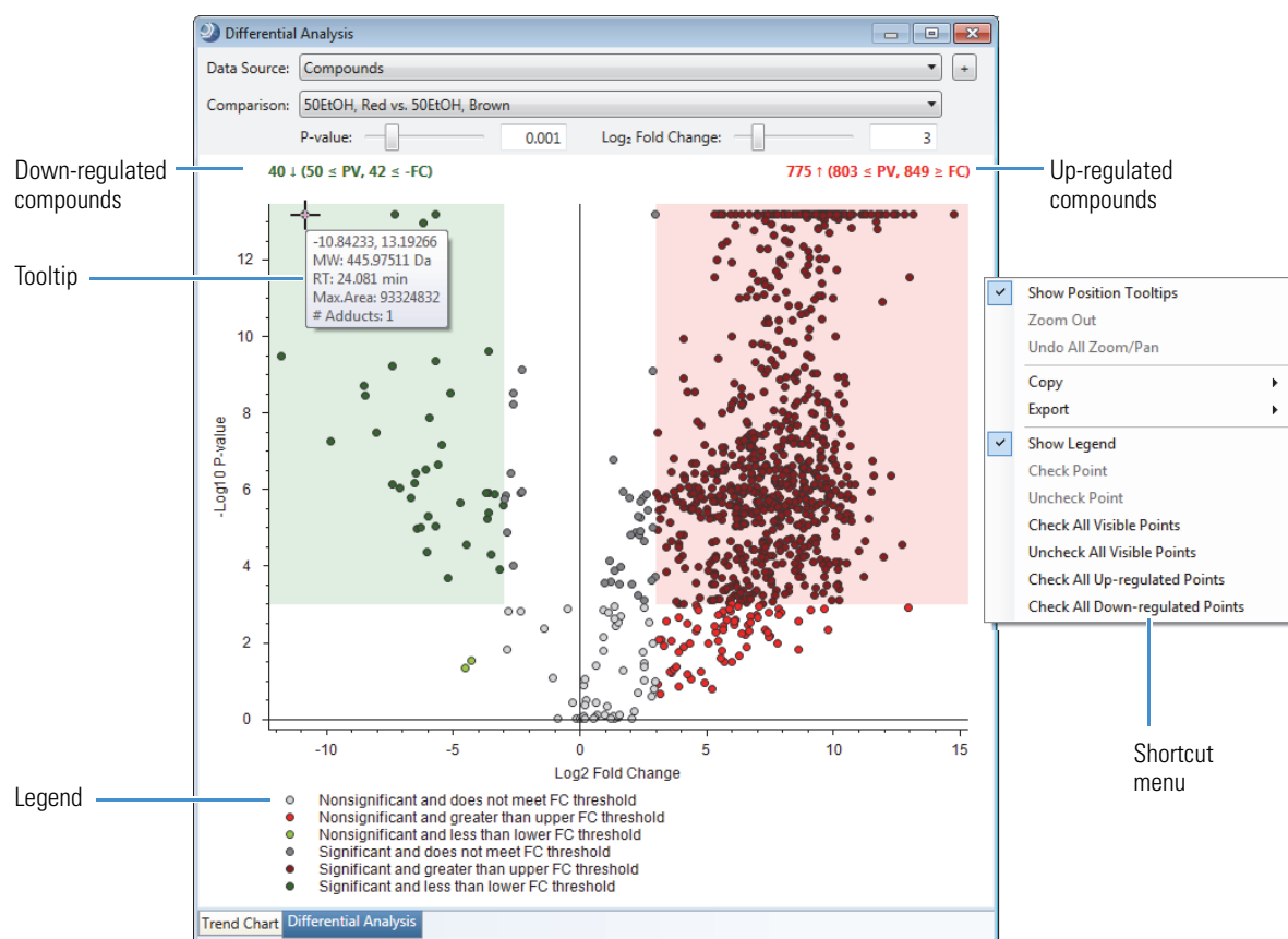
Figure 8. Differential analysis for the compounds extracted from red o-rings or brown o-rings with 50% ethanol/water
