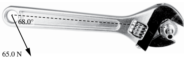
FIGURE 5.11 An acting force that is not perpendicular to the lever arm of the object will also generate a torque.
