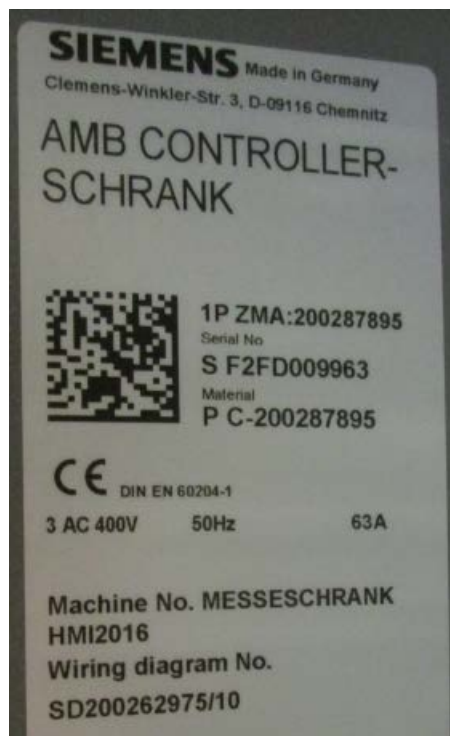
Figure 6-59 Example: Nameplate for control panel
