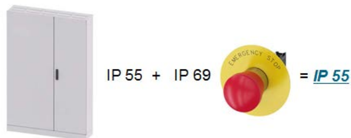
Figure 6-75 Example: Alteration of the degree of protection by installation of a component
