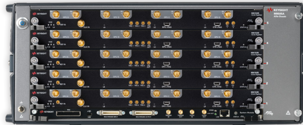
Figure 2. Five M9703B AXIe 12-bit digitizers installed in the M9505A 5-slot AXIe chassis to form a 40-channel 12-bit acquisition system.
