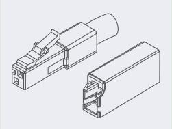
Type 1 SPE Connector IEC 63171-1 | Copper LC Connector
