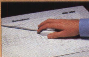
MM digitizers are available with either cursor or pen-like stylus.
