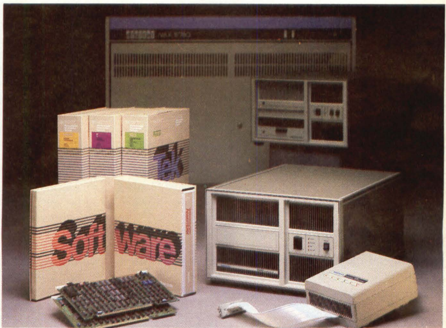
Figure 1: Tektronix Microcomputer Development group supports cross-development on the Digital Equipment Corp. VAX-11 series computers with compilers, linkers and loaders. Final hardware and software integration as well as software debugging occurs with the dedicated resources of the 8540 integration unit and associated in-circuit emulators.
