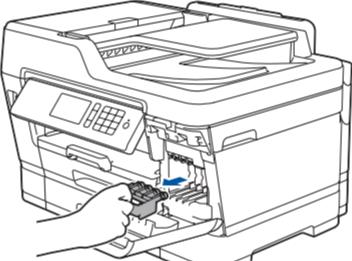
Open the ink cartridge cover and remove the orange protective part from the machine.
