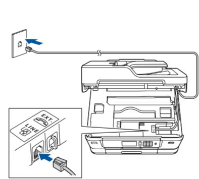
Connect the telephone line cord. Use the jack marked **LINE** and guide the cord out the back of the machine.
