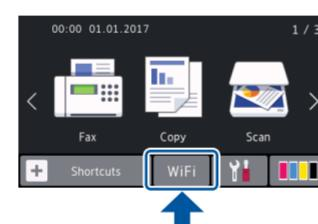
Select the SSID (Network Name) for your access point/router and enter the Network Key (Password).
