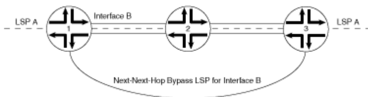
Figure 19: Node Protection Creating a Next-Next-Hop Bypass LSP
