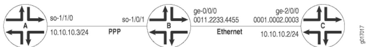
Figure 120: Sample Topology of Layer 2.5 Translational Cross-Connect
