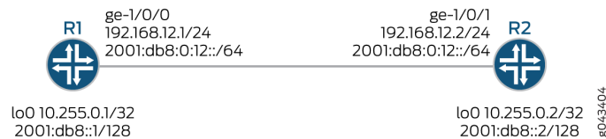
Figure 93: Example LDP Native IPv6 Support
