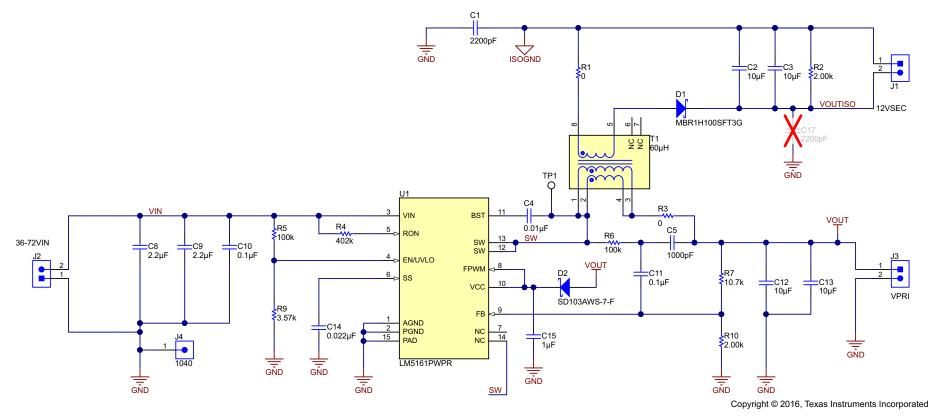
Figure 10. Fly-Buck EVM Schematic with the LM5161 IC
