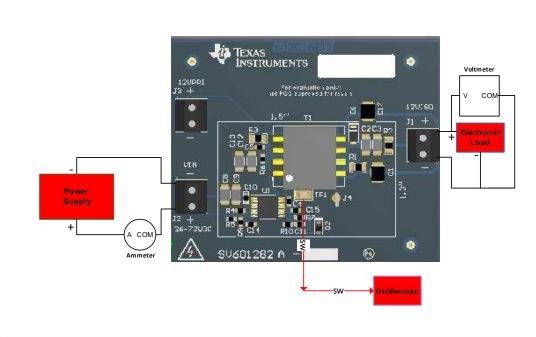
Figure 1. EVM Test Setup
