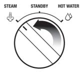
Rotate the STEAM/HOT WATER dial to the HOT WATER position and run water through the hot water outlet for 10 seconds.
