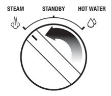
Descale Hot water component by turning the steam dial to the RIGHT towards the HOT WATER icon.
