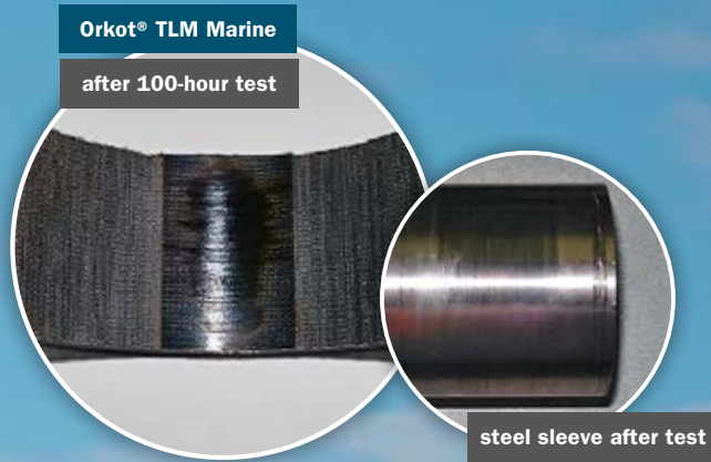
No damage has been caused to the sleeve. The scar on the sleeve was already present from previous tests.
