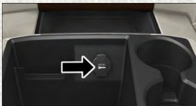
Power Outlet — Center Console
