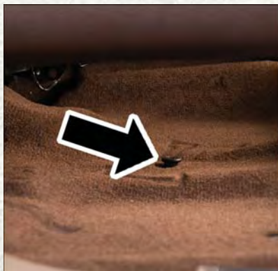
Floor Fastener Location
