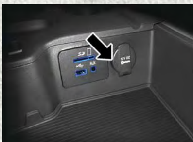
Power Outlet — Storage Compartment
