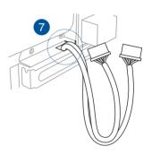
9. Connect the passive fan module cables to the cables located inside the chassis.
