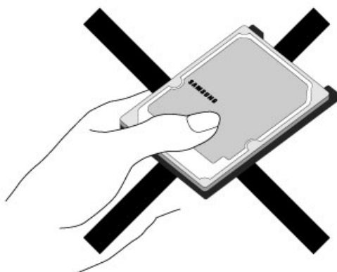
Fig. 7-2: HDD handling guide~Do not Touch Cover and PCB!
