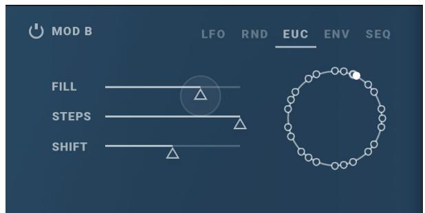
For example, in a 16 step sequence a 25% fill will result in 4 distributed gates.
