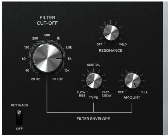
Even if a source, or a blend of sources, sound fantastic on its own, a synth bass sound is all about how you filter it, and how the filter changes when you hit a note. We want to make that as easy as possible and boiled it down to four main controls: the four knobs to the right.
