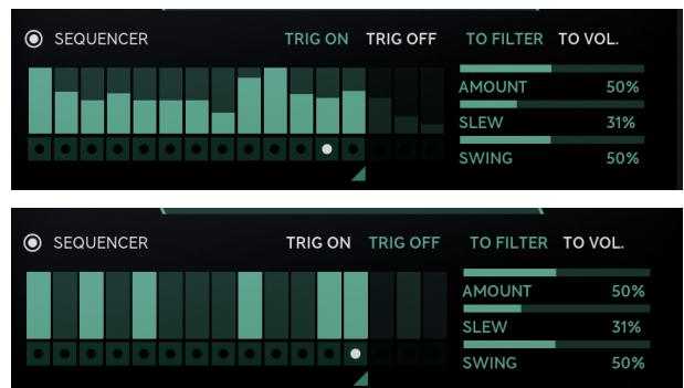
**Seq On/Off** This small button at the upper left of the Sequencer window enables or disables the sequencer. When turned off, the sequencer window is blacked out.
