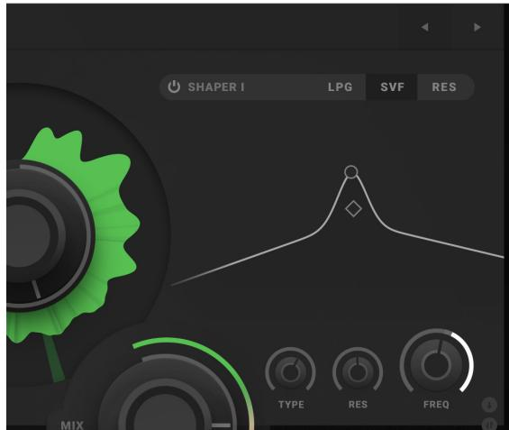
3. Click on the other hotspot in the filter diagram and try to move it. You'll notice that it is linked to the Type knob and locked to be modified only horizontally. When the Type parameter is changed from a low value to a high value, the SVF topology is seamlessly changed from a lowpass filter, on to a bandpass filter and finally a high pass filter. The displayed graph also reflects this behaviour.
