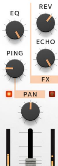
**EQ** Boosts or cuts the frequency range where most of the hi-hat's tonal content is found. The neutral setting is at 12 o'clock, turn counterclockwise to cut this frequency range (emphasizing the noise character) and clockwise to boost (emphasizing the tonal character).
