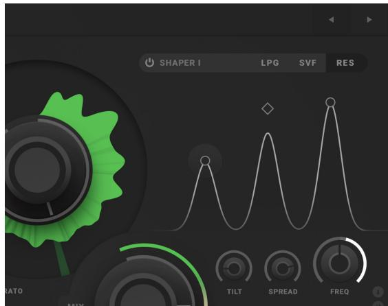
5. Let's click on the hotspots on one of the side-peaks in the filter curve. Clicking and dragging your mouse or touchpad reveals that moving the side-peaks hotspots vertically changes the RES Tilt (peak emphasis), while moving them horizontally changes the RES spread (the space in frequency between the different peaks). This change is, of course, also reflected on the adjacent knobs on the lower middle and left in the Shaper section.
