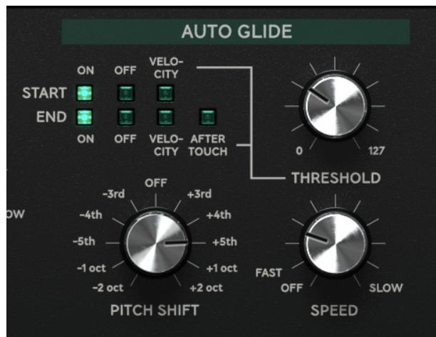
**Auto Glide Start** This parameter determines whether the glide will occur in the start of the sound. When set to the velocity option, the threshold-level will determine at which velocity the auto-glide is triggered.
