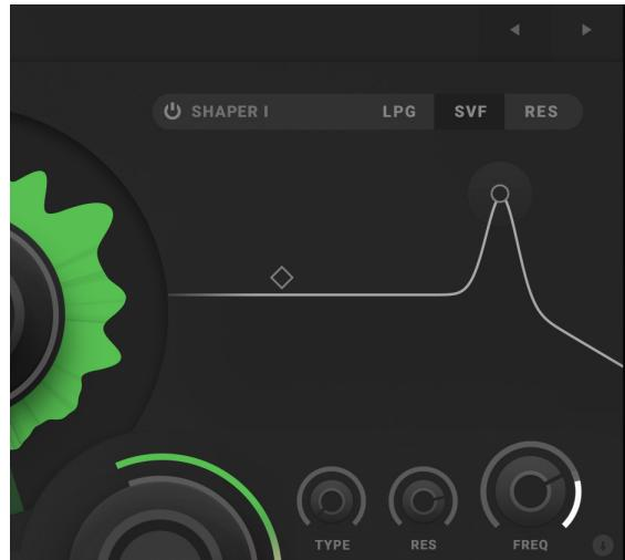
2. Now try clicking on the hotspot in the displayed SVF (state variable filter) curve - it's on the crest or peak of the curve. Try clicking and moving it around while playing. You'll notice that by changing this graph in horizontal direction changes the SVF cutoff frequency while changing the graph in vertical direction changes the SVF resonance. Note also that the cutoff frequency and resonance knobs changes with the curve and vice versa.
