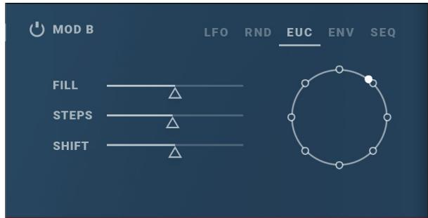
**EUC fill (0-100%)** This parameter determines how many percentage of the available steps in a bar that will send gates.
