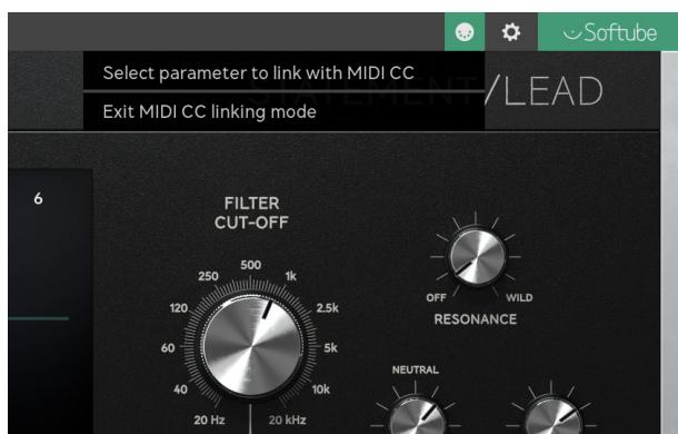
After entering MIDI CC linking mode, the on-screen message will prompt you to “select parameter to link with MIDI CC” and this means that you can click on any parameter you would like to link to your controller.
