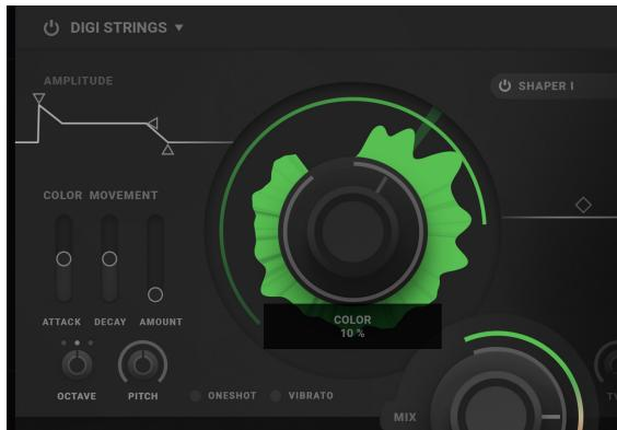
3. Turn down the upper Source Movement Amount slider to zero. Now try to move the big Color knob clockwise and counterclockwise back and forth while playing. You will notice that the sound goes from a duller string sound to brighter one the further clockwise you will go. And at the very end the waveform is silent.
