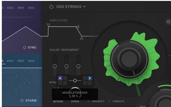
6. As we noticed before, when the modulation mix slider is set somewhere in the middle, in between the modulation source selected on the left and on the right, the modulation color is white; indication that there is a mixture of two modulation sources going on here.
