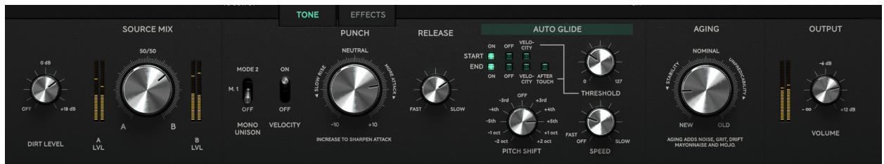
Next step is to adjust the shape, the envelope, of the tone. That's easily done by adjusting the Punch control. Increase Punch and you'll get a snappier, punchier sound. Decrease it and you'll get a sound with a slow build-up. The Release sets the time it takes for the sound to fade-out.
