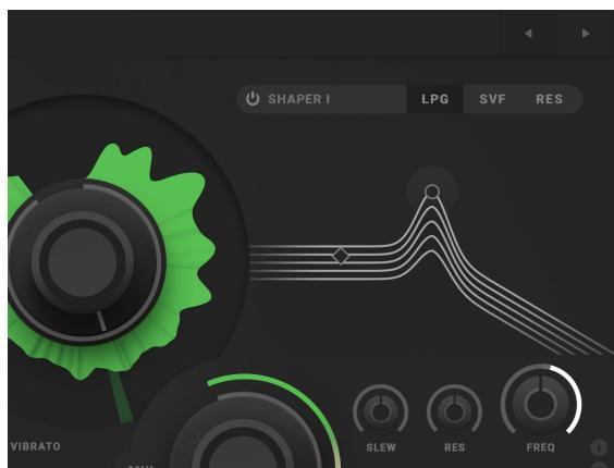
6. At last, let's look at the Shaper LPG mode. LPG stands for Low Pass Gate which is a special vactrol-controlled filter and VCA combination controlled via a so called vactrol, often used in so called West-Coast modular synthesis. Parallels's Shaper LPG mode draws some inspiration from the classic LPG to create a filter with a controlled "sloppy" cutoff response. Click on the LPG tab on the Shape mode selector on the top right to bring up the LPG filter curve.
