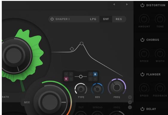
7. As pictured and described, you can route any modulator to any destination by clicking on the other ring of a parameter of choice. Then chose the modulation from two of the four modulation slots and the mix balance between them. Set the amount of modulation at the destination by clicking on the other ring of parameter again, and drag your mouse or mouse-pad upwards (the ring around the parameter will fill up).
