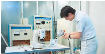
Test using an electrostatics tester
