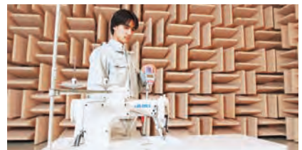
Noise rating in a semi-anechoic chamber
