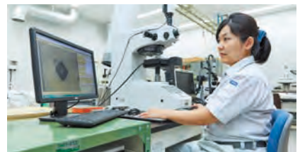
Hardness test using a Vickers hardness tester
