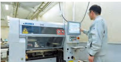
Durability test for a chip mounter
