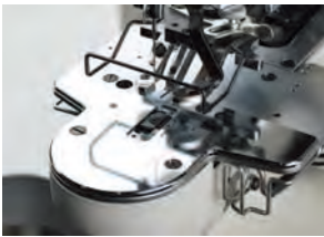
Mechanism for shorter remaining thread in the LK-1903BB
