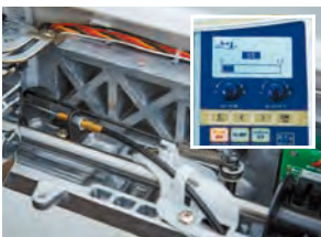
Controlling the presser height for the HZL-EX7
