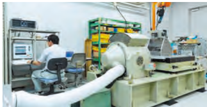
Vibration test using a vibration exciter
