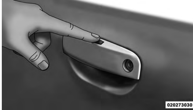
Push The Door Handle Button To Lock
