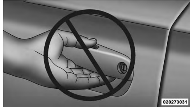
Do NOT Grab The Handle When Locking
