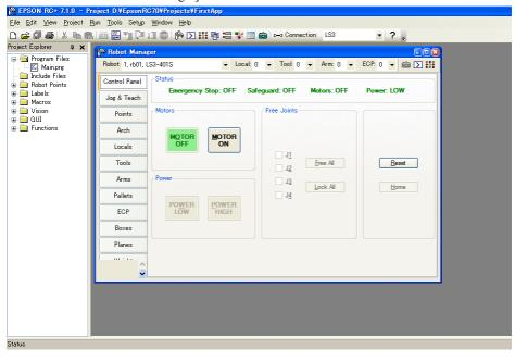
(2) Click the [Control Panel] tab. Then, click the <Motor On> button to turn on the Manipulator motors. You will be prompted to confirm the operation.
