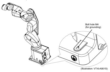
For DC specification Manipulator, connect the ground and DC power wire (-).
