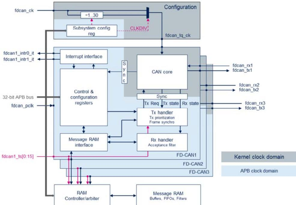
The CAN sub-system supports 3 FD-CAN controllers named FD-CAN1, FD-CAN2 and FD-CAN3.
