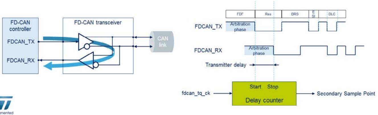
The transmitter delay compensation enables configurations where the data bit time is shorter than the transmitter delay.
