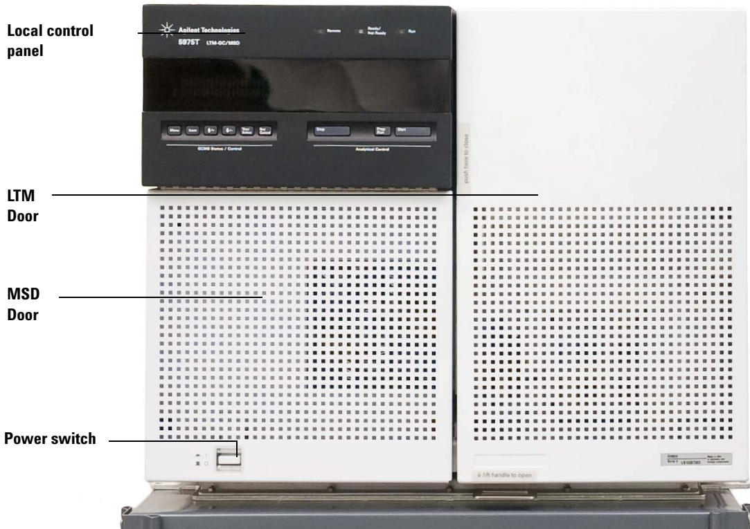
Figure 1 5975T LTM GC/MSD system
