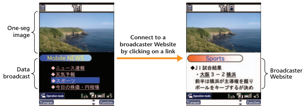
Figure 4 Linking between BML browser and i-mode
