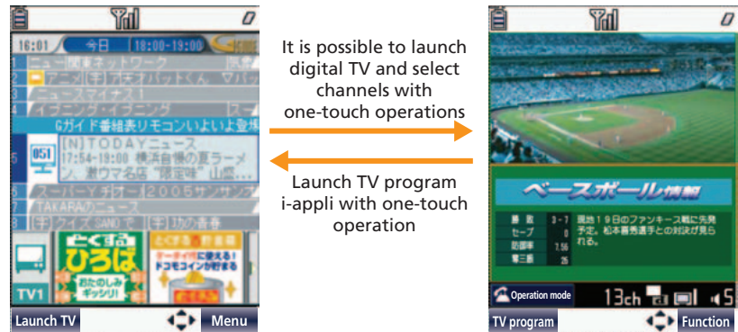
Figure 6 Linking between TV program i-appli and one-seg launch
