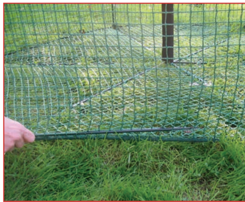
5) Connect each of the 6 rail strengthening bars by weaving each bar through the netting along the top and bottom of unit and connect to the 2 vertical posts on each corner
