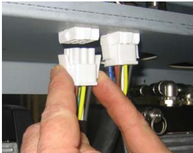
Fig. 9-15 – disconnect multi-pin plug
