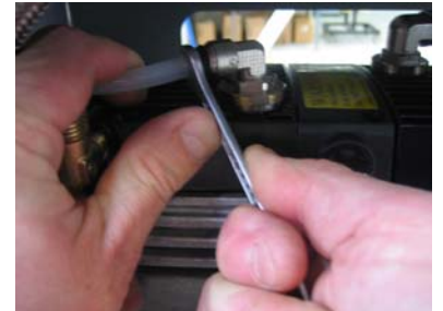
Fig. 9-14 – pull away pipe
