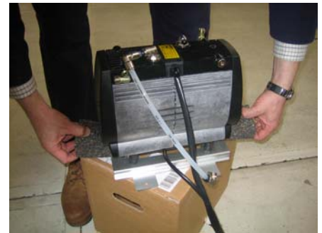
Fig. 9-17 – remove transit support blocks
