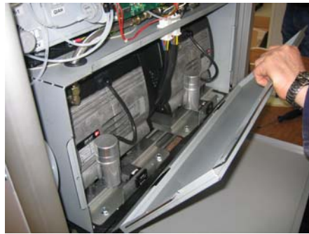
Fig. 9-10 – remove second cover
