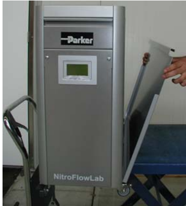
Fig. 9-9 – unscrew side panels
