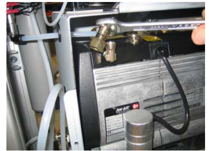
Fig. 9-11 undo bull nose connections
