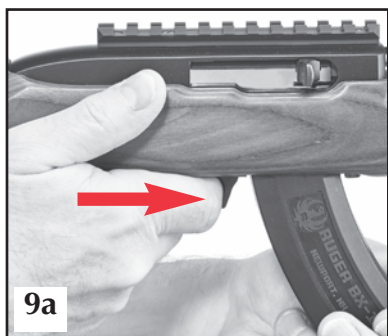
Figure 9. The safety should be “on” when the magazine is being removed or inserted. Move the magazine release forward (Figure 9a) and draw the magazine out by grasping it between your thumb and forefinger and draw it out of the gun (Figure 9b).
