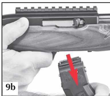
Figure 9. The safety should be “on” when the magazine is being removed or inserted. Move the magazine release forward (Figure 9a) and draw the magazine out by grasping it between your thumb and forefinger and draw it out of the gun (Figure 9b).
