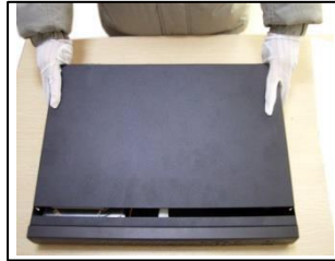
② disassemble the cover
