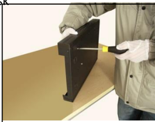
④ fix the screw of hard disk
