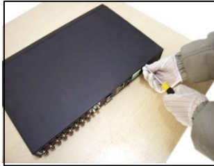
① disassemble the screw
