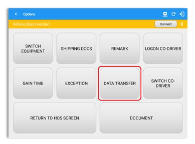
Tap the *Data Transfer* button to transfer data of the compilation of the driver's ELD records. Once tapped, a selection of the supported data transfer options by the ELD will prompt to the user. The available data transfer options for iOS app are Bluetooth, Email and Web Service only.
