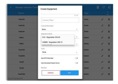
A *Regulation Mode* option to switch between 395.15 (AOBRD) and 395.20 (ELD) support is available. When 395.15 (AOBRD) mode is selected it turns off all 395.20 (ELD) features. It simply records the drivers' events regardless to the FMCSA rules. ELD is set as the default regulation mode for all new equipment.
