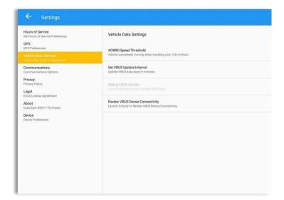
Also, drivers have the ability to set speed threshold on the app->Vehicle Data Settings->AOBRD Speed Threshold only if the driver is allowed. To allow a specific driver, enable the option which can be seen in portal->Drivers Management Page->Set AOBRD Speed Threshold option.
