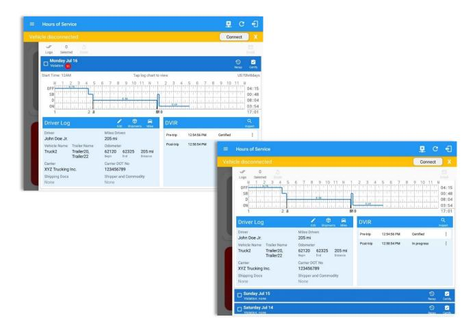
Scroll the screen to view all of the information, or, tap the log grid to view the log events. The daily log for the current day will be in expanded view by default. The daily driver logs for the previous days will be in collapsed view.
