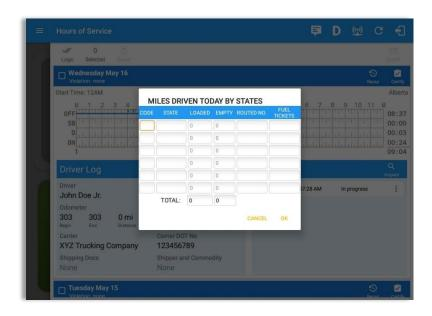
Tap the *Miles* button to open the *Miles Driven Today by States* dialog. This is where you can fill in the shipment data that is required to be included in the driver's daily log. Required data includes:
