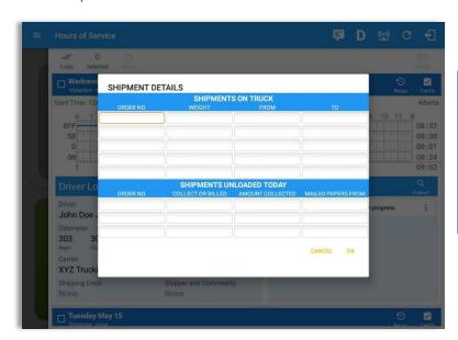
Tap the *Shipments* button to open the *Shipment Details Form*; you can fill in the shipment data that is to be included in the driver's daily log.
