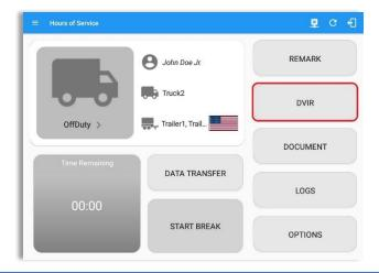
From the *Hours of Service Main Screen*, tap the *DVIR* button to display the *DVIR* screen.
