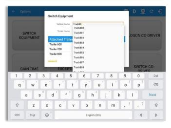
Select the **Vehicle ID** or **Trailer ID** dropdown list and select the required vehicle or trailer, then tap the **Switch** button to switch to the selected vehicle or trailer.
