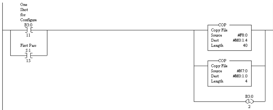
Figure 6.2 Typical Ladder Program
