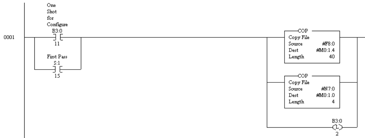
Figure 7.2 Typical Ladder Program
