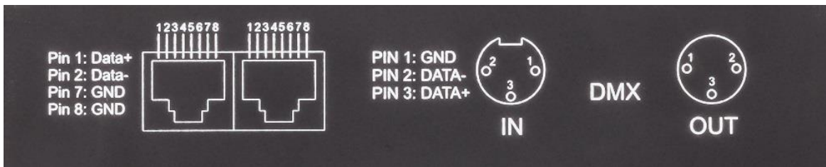
Figure III: Connector Pinout for DMX-4-5000-3-10A
