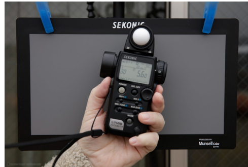
Figure 18 The cinematographer uses a light meter and an 18% gray chart to set camera exposure
