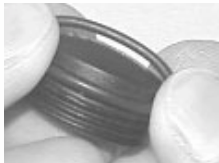
Fig. 119 - TRANSMITTER O-RING INSTALLATION
