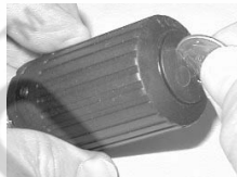
Fig. 118 - TRANSMITTER BATTERY COVER REMOVAL
