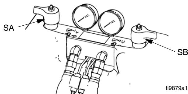
4. For models with a dispense valve with a safety lock, engage gun safety lock.
