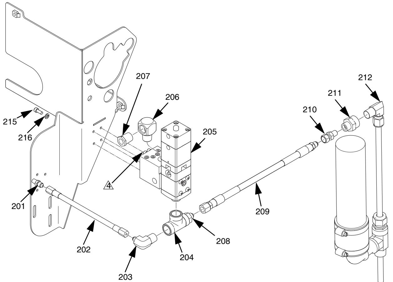
2- Apply pipe sealant to all male threads as needed prior to assembly.
