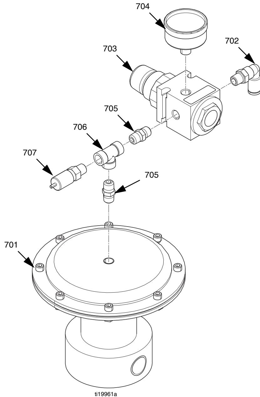
1. Apply pipe sealant to all male threads prior to assembly.
