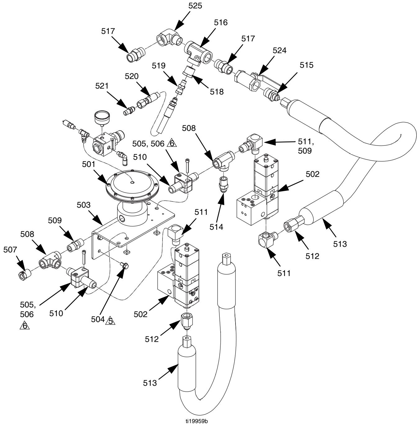
2. Apply Sealant to all male threads prior to assembly.
