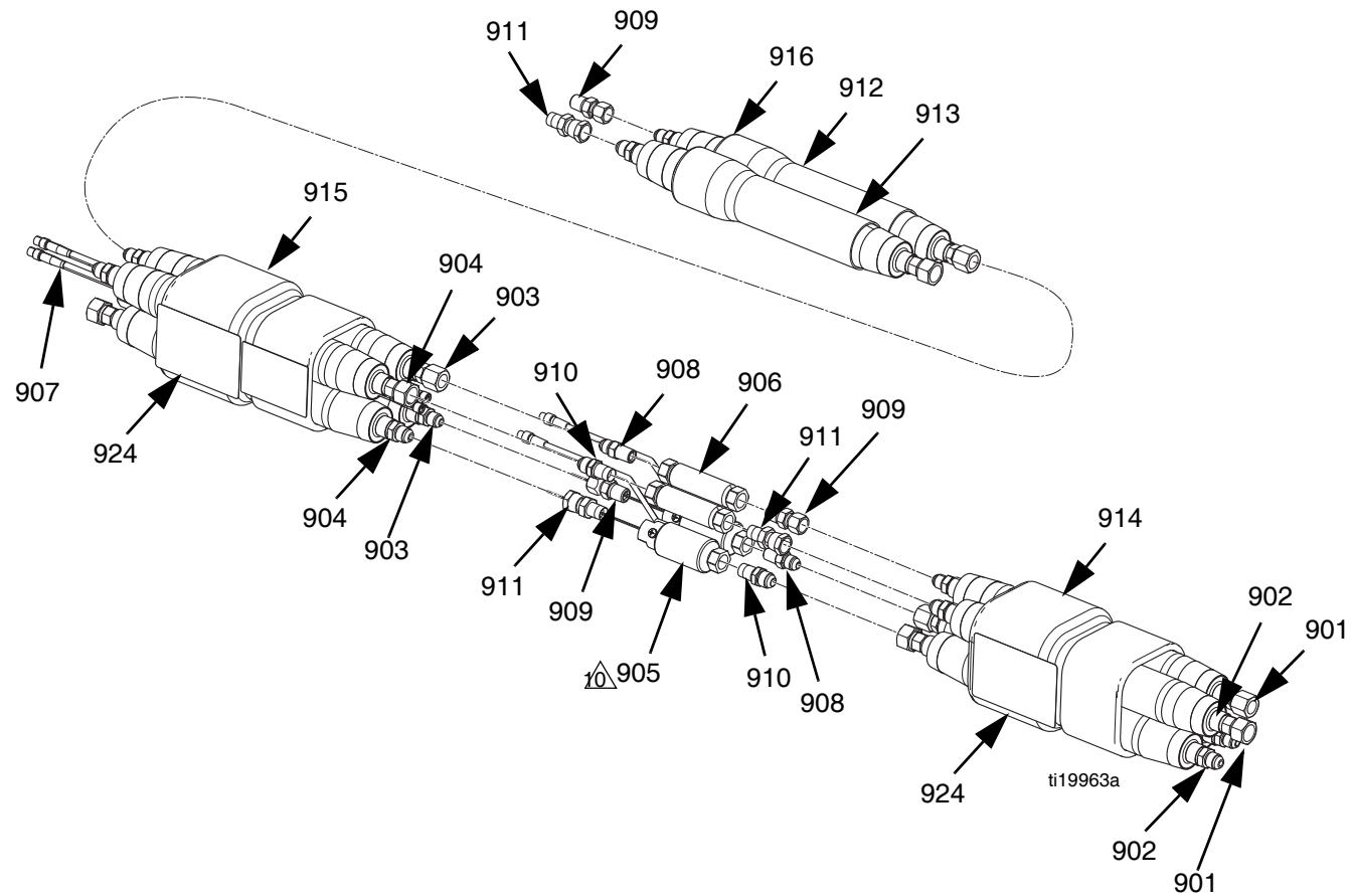
9- Apply pipe sealant to all male threads as needed prior to assembly.
