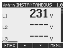
Figure 3-3 Display of the measured voltage in the case of connection type 1P2W
