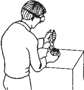
HEAVY DIAGONALS ARE FINE FOR CUTTING THE SPREAD ENDS OF COTTER PINS.
