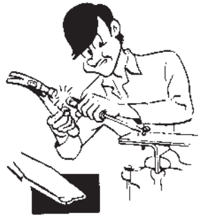
Fig. 6-14. Never use a screwdriver as a chisel.
