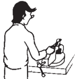
DON'T USE FLAT NOSE PLIERS TO PRY OR TWIST.
