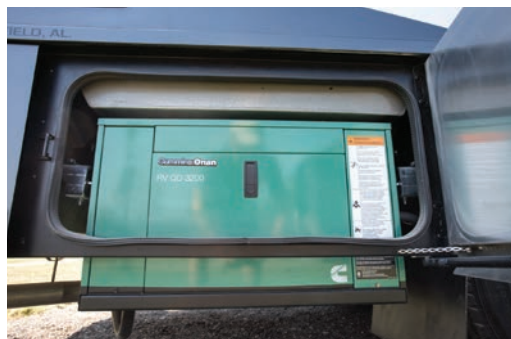
From far left: The exterior TV, concealed behind a flush-mounted door, allows easy viewing from the patio. A 3.2-kW diesel-fired generator provides power on the road or in locations where hookups are not available.
