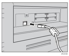
Connect the other end of the Ethernet cable to a network connection device such as a hub.
