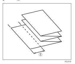
This menu appears only when the folding finisher is installed. The default setting is **40 mm** (Metric version) / **1.50 inch** (Inch version). Use the number keys to enter a value in 1 mm units in the ranging from 35 mm (1.00 inch) to 40 mm (1.50inch).
