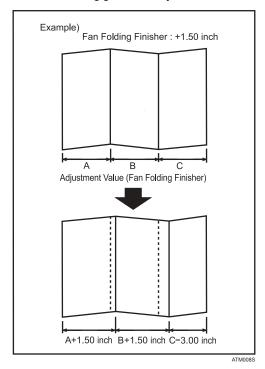
The default setting is 0.0 mm (Metric version) / 0.00 inch (Inch version). Enter a value in 0.5 mm units in the ranging from -6.0 mm (-0.24 inch) to 6.0 mm (0.24 inch).
