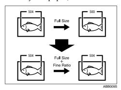
The default setting is Vertical: **0.0**% / Horizontal: **0.0**%. Specify the ratio between –1.0% and 1.0% (in 0.1% increments)
